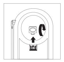
3. Put the retainer back into its slot on the Base Unit.
